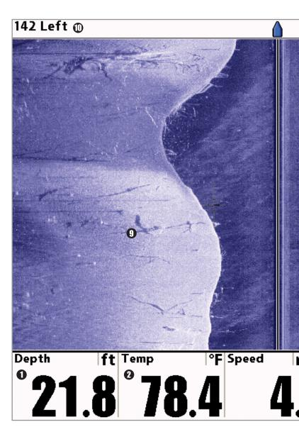
ate interpretation of bottom contour and structure. For Side Imaging, the bottom composition determines the intensity of the sonar return. For example, relative density. Upward slopes that face the transducer reflect sonar better than downward slopes that face away from the transducer. You can find or accurate interpretation of bottom contour and structure, including the following items:
